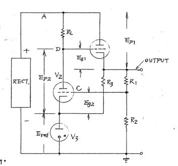
In this circuit, it is necessary to maintain Ep2 at least more than 10 volts so as to enable voltage amplification within tube  $V_2$ , and Eg1 should vary down to a voltage to cutoff regulator tube  $V_1$ . Therefore, in regulated power supplies with low voltage outputs, voltage at point C is made as low as zero or negative.
